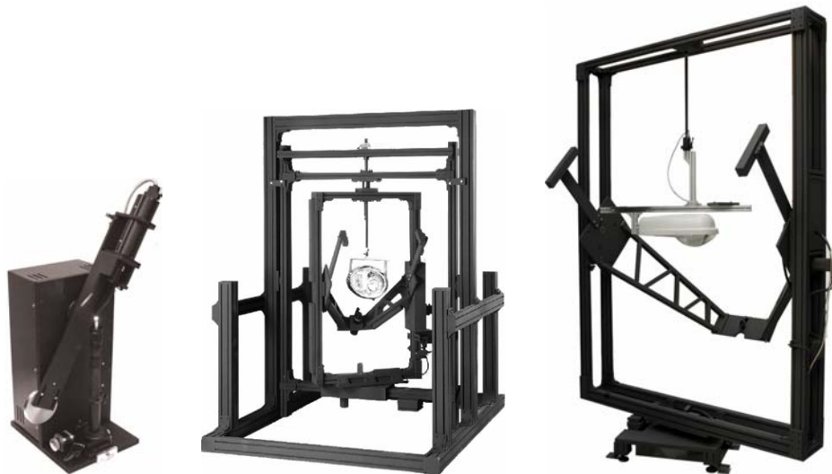
Abbildung 4: LED – Goniophotometer, schwenkbares Lampengoniophotometer, Leuchtgoniophotometer
