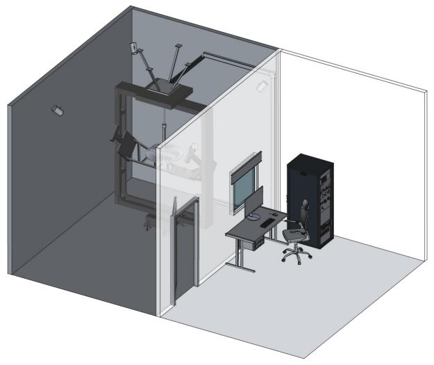
The upper fixation point of the goniometer is secured via a ceiling-mounted brace, ensuring stable fixation.
