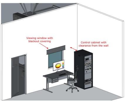
cable routing. Additionally, sufficient clearance must be planned behind the cabinet to allow unobstructed access to the rear door.
