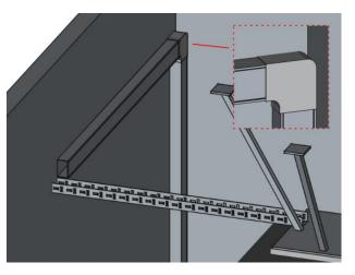
nel (Adam Hall, Defender NANO BLK) to the rear wall. From there, a  $60 \times 60$  mm cable duct continues the routing toward the partition wall of the control room.
