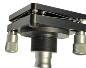
Figure 9: Leveling unit of the test fixture
