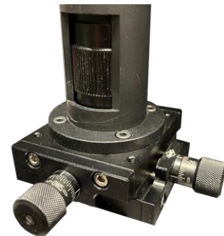
Figure 8: X/Y adjustment unit and Z fine adjuster
